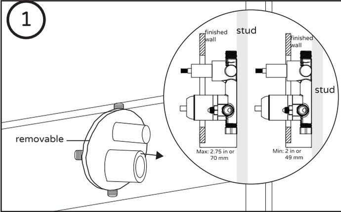
Confirm the installation position and remove the plaster guard. NOTE: Plaster guard surface must be flush with finished wall surface (tile, etc).
