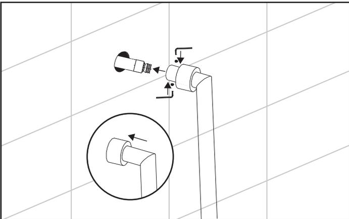
Slide top pipe onto inlet fitting (3) and secure with set screw (2). Slide escutcheon (4) to cover set screws
