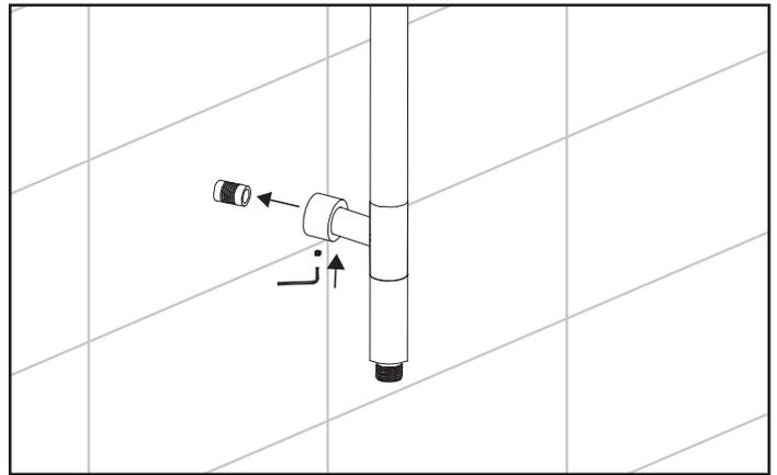
Slide bottom support over bottom mount (9) and secure set screw (2).
