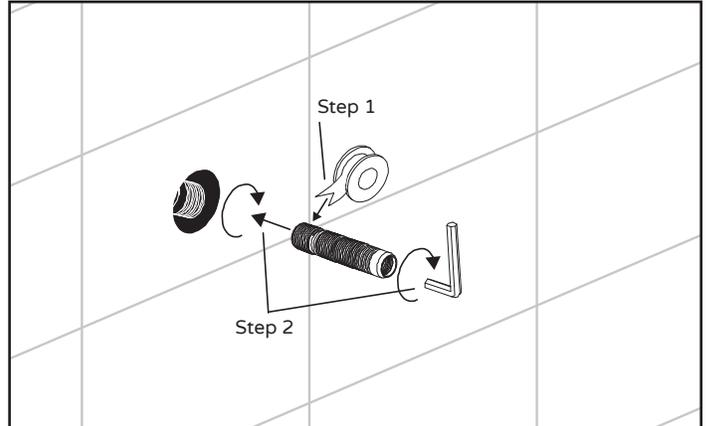
Screw nipple extension (5) into pipe. Make sure you have 1/2" off the wall.
