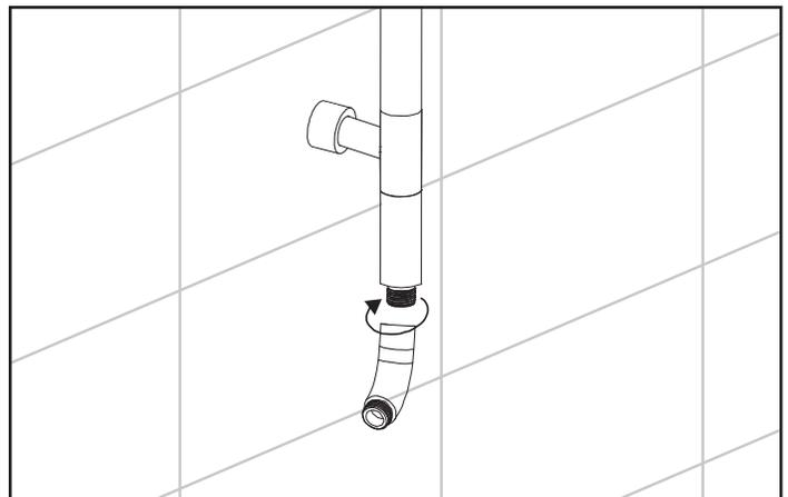
Screw swivel joint (7) onto shower bar.
